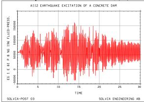
Dam water pressure 12 m below surface, (Pa).
